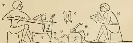
Carpenters. (Wilkinson.) r, drills a hole in the seat of a chair; s, t, legs of chair; u, u, adzes; r, a square; r, man planing or polishing the leg of a chair.
